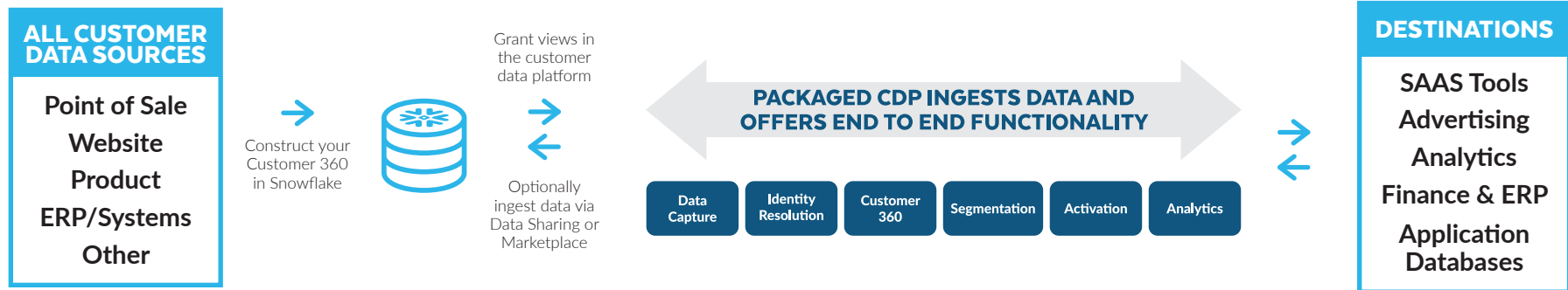
Figure 1: Example of a high-level architecture of a composable CDP powered by Snowflake.
